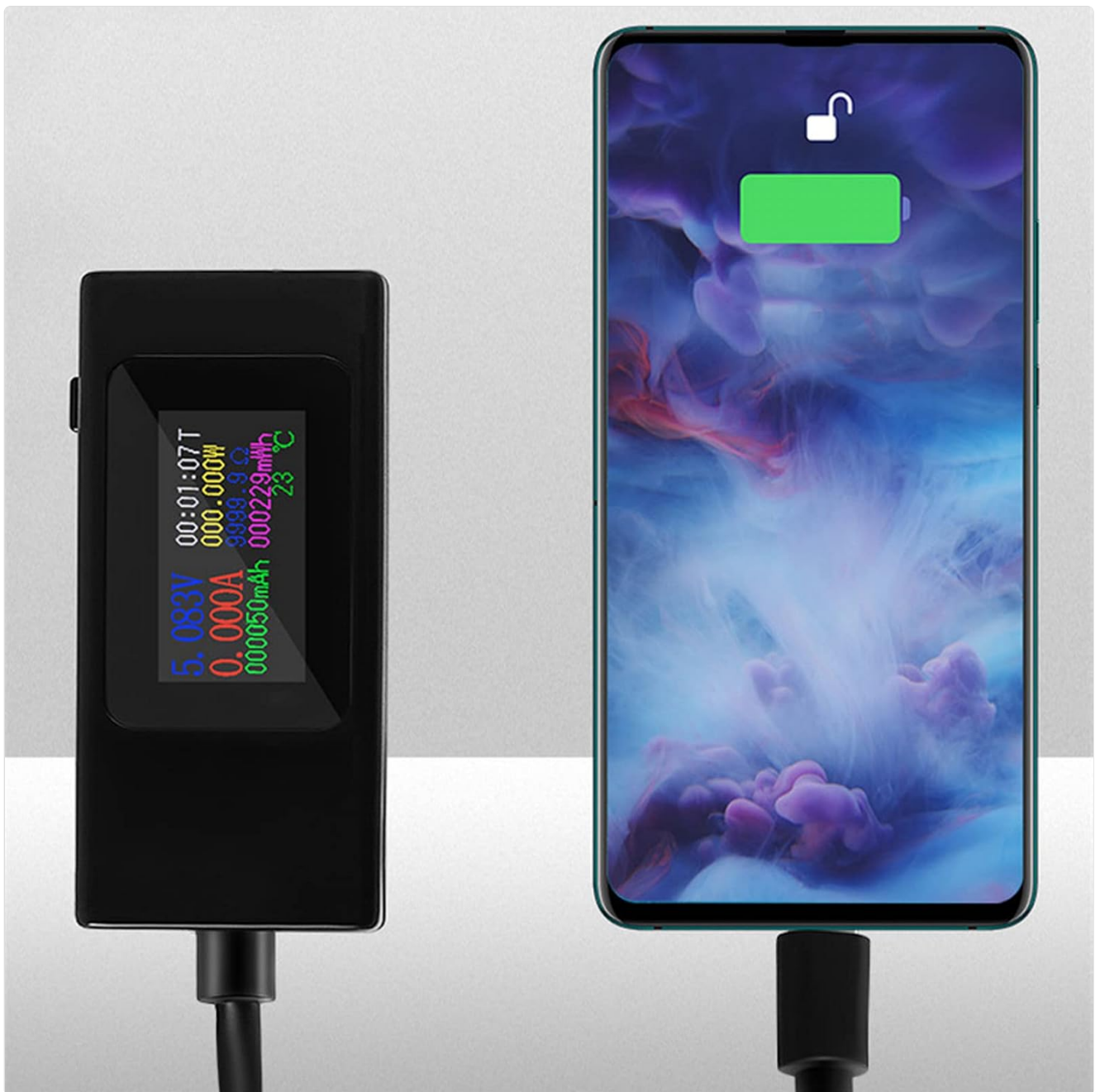
Figure 4.2: The tester connected in-line, measuring power delivery to a smartphone.
