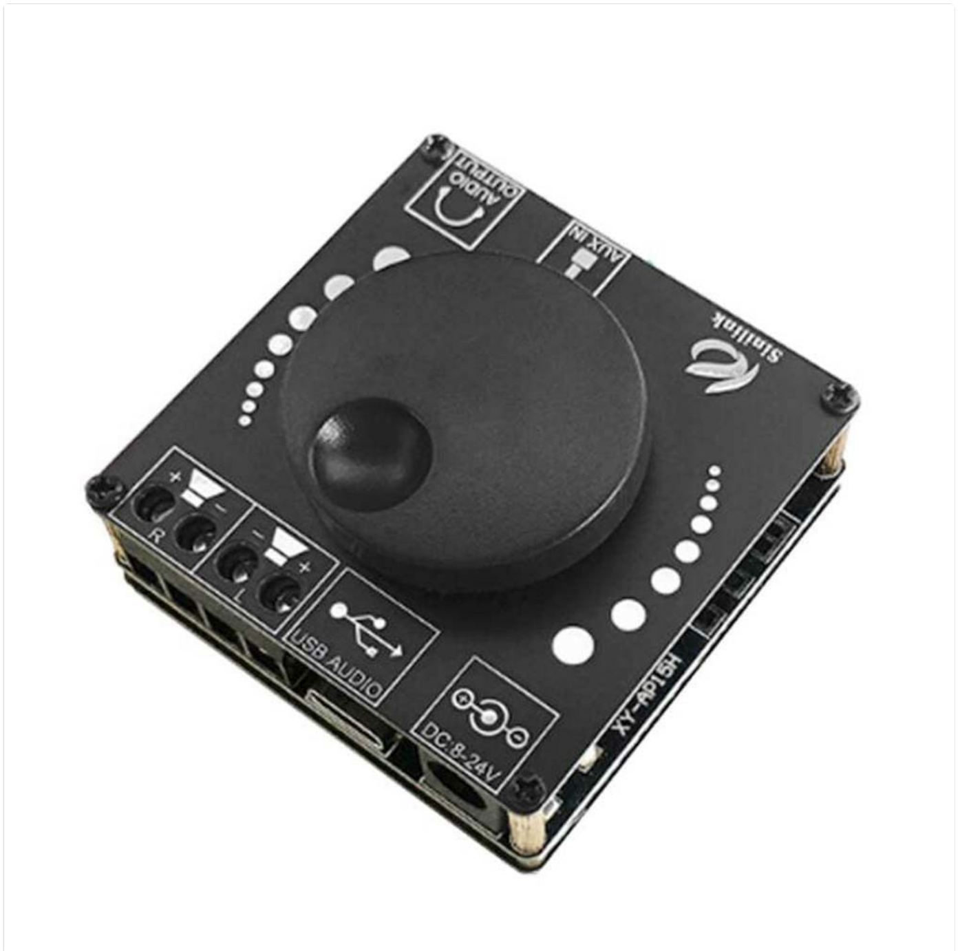
Figure 3.1: XY-AP15H Amplifier Board Layout. This image displays the top view of the amplifier board, highlighting the main volume knob, AUX In port, USB Audio port, DC power input (8-24V), and stereo audio output terminals (R and L).
