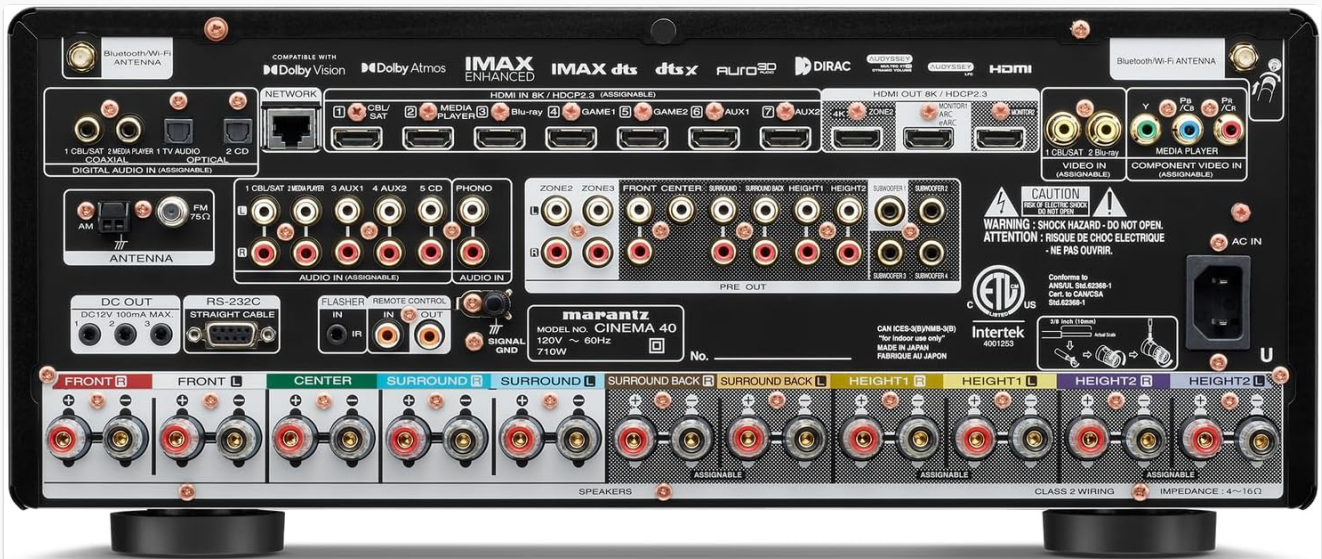
Figure 4.2: Rear view of the Marantz Cinema 40 Receiver, illustrating the comprehensive array of input and output ports, including HDMI, speaker terminals, and network connections.
