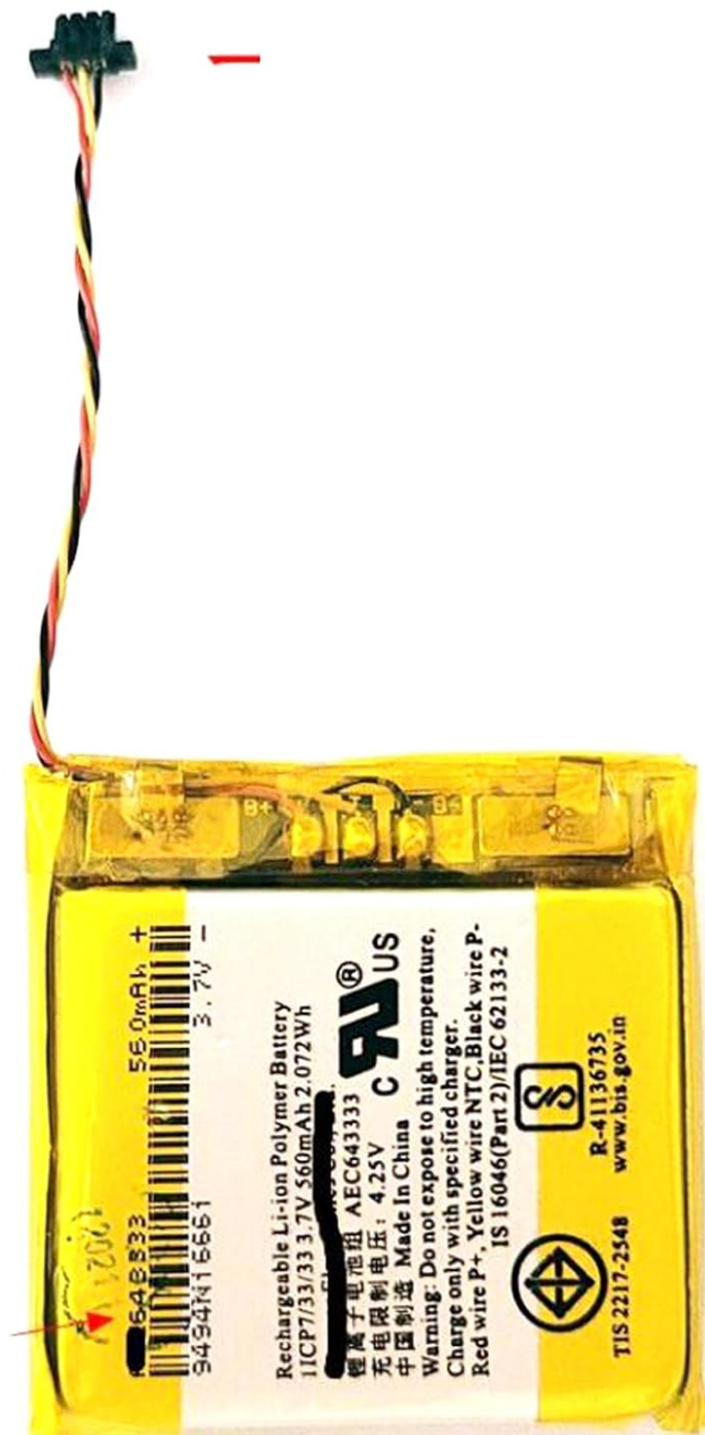
Image 3: A clear view of the JINWEI AEC643333 battery, emphasizing its compact size and the small, multi-pin connector at the end of its wires, crucial for connecting to the headphone's internal circuitry. The part number 9494N16661 is visible on the label.
