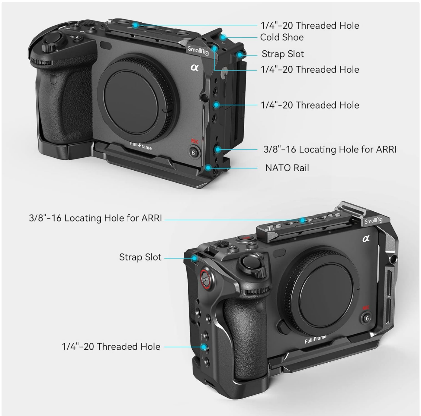
Figure 4.1: Detailed diagram illustrating the multiple mounting points available on the cage, including threaded holes, cold shoe, ARRI locating hole, and NATO rail.
