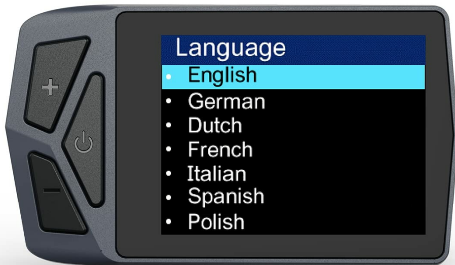
Figure 5.3: Language selection interface on the B02N display. This image shows the display screen presenting a list of 8 language options for user selection.
