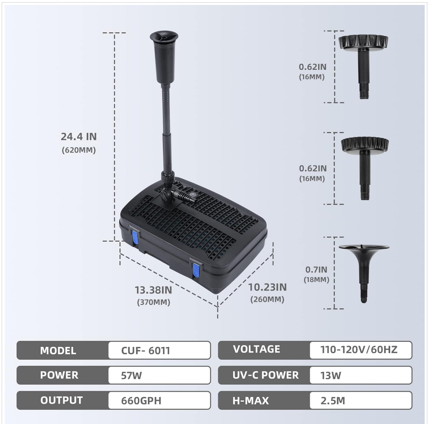
Image: A diagram showing the physical dimensions of the Anbull CUF-6011 pond filter system and a table summarizing its key specifications.
