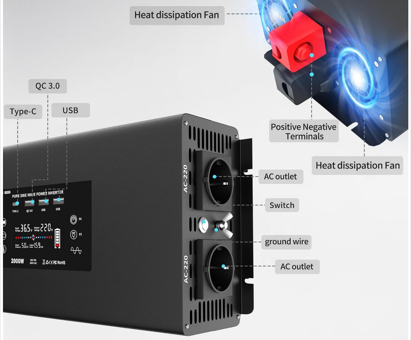
Figure 2: Detailed view highlighting the inverter's components. This image shows the heat dissipation fans, positive and negative terminals, AC outlets, switch, and ground wire connection points. The front panel includes Type-C, QC 3.0, and standard USB ports.
