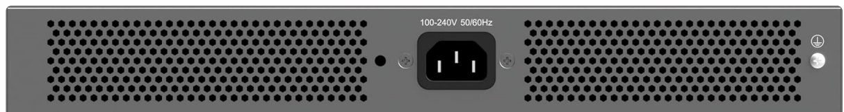
Image 4: Close-up of the rear power input (100-240VAC, 50/60Hz) on the Grandstream GWN7801P PoE Switch.
