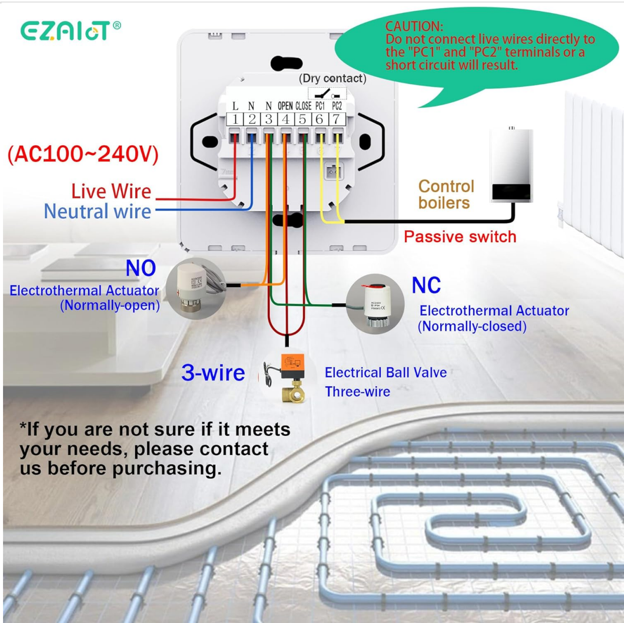
Image 2: Wiring Diagram. This detailed diagram illustrates the wiring connections for the EZAIOT Smart WiFi Thermostat. It shows connections for Live (L) and Neutral (N) wires (AC100~240V), and terminals for controlling boilers via a passive switch. Connections for Normally Open (NO) and Normally Closed (NC) electrothermal actuators are depicted, along with a 3-wire connection for an electrical ball valve. A critical warning advises against connecting live wires directly to 'PC1' and 'PC2' terminals to prevent short circuits, emphasizing the importance of correct installation.
