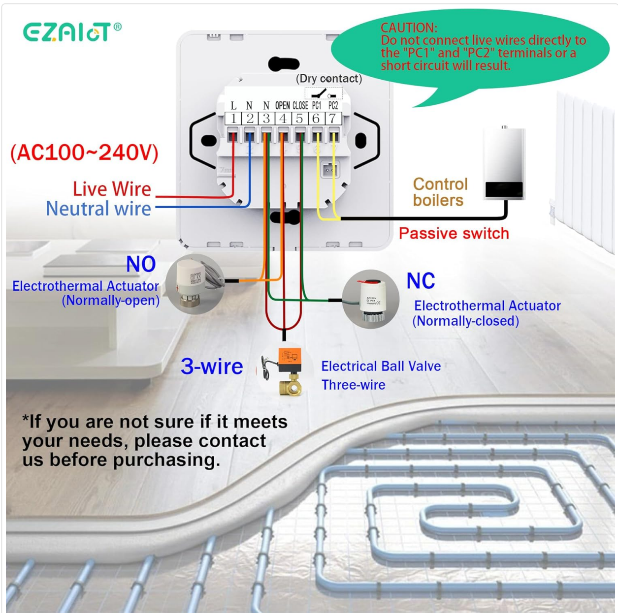
Image 4.3: Detailed wiring diagram for the EZAIoT Smart WiFi Thermostat, illustrating connections for live wire, neutral wire, control boilers (passive switch), and electrothermal actuators (normally-open and normally-closed).
