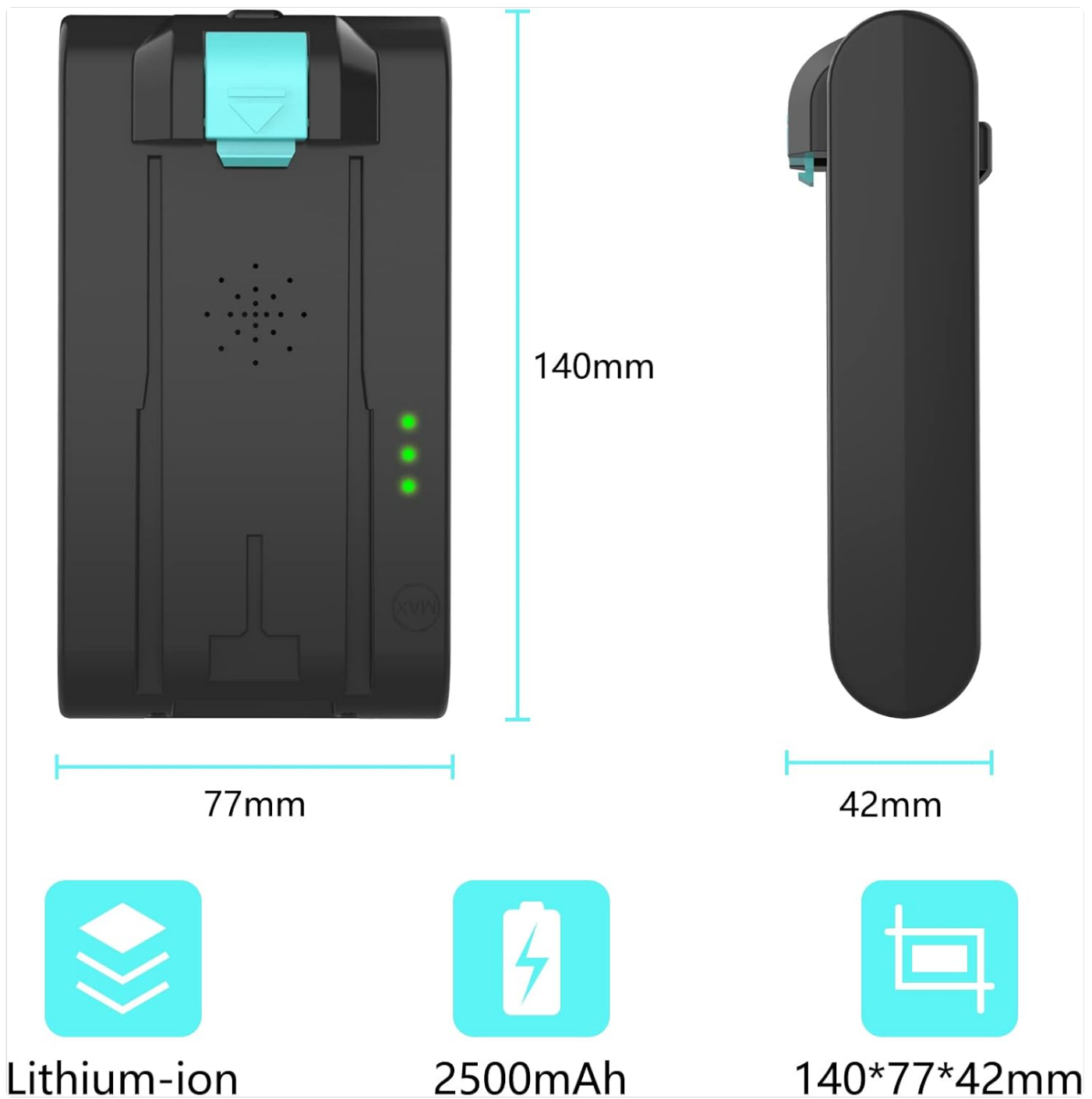
Figure 2.2: Dimensions of the WOWGO S108B Replacement Battery. The battery measures 140mm in length, 77mm in width, and 42mm in height. Key specifications like Lithium-ion, 2500mAh capacity, and dimensions are highlighted.
