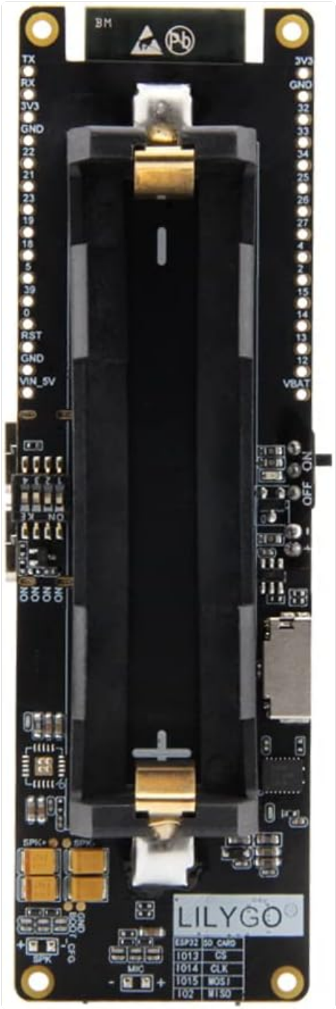
Figure 3: Top view of the board highlighting the 18650 battery holder and surrounding components.
