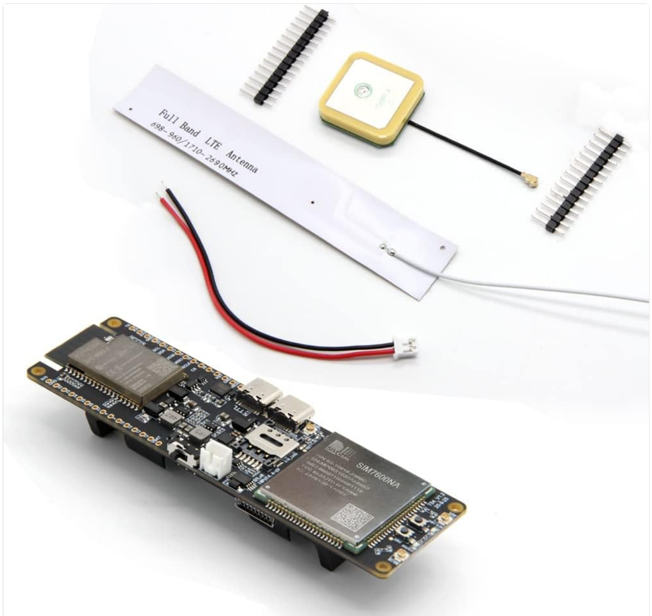
Figure 2: The LILYGO T-SIM7600NA board along with its typical accessories, including LTE and GPS antennas and pin headers.
