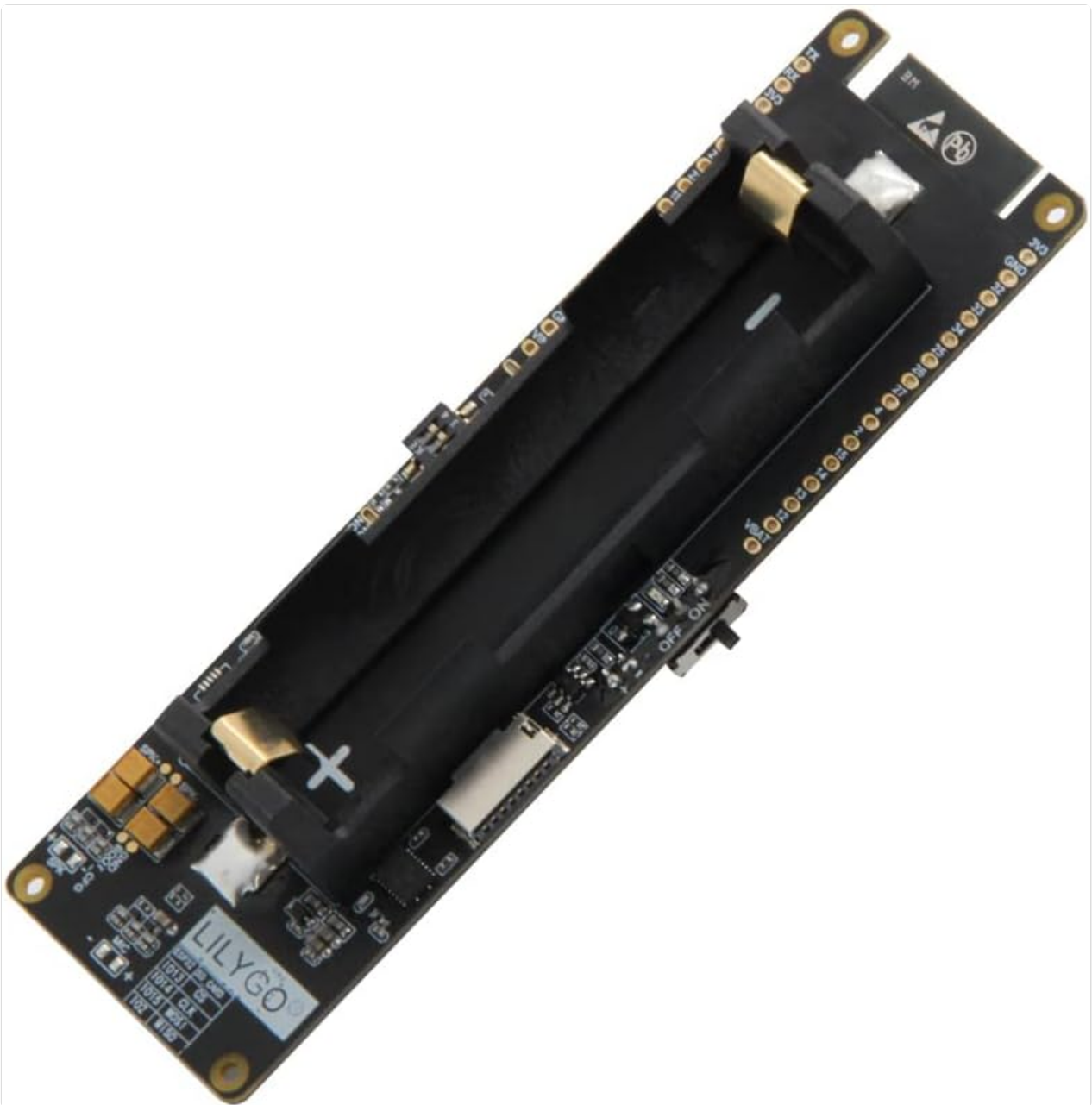
Figure 4: Angled view of the board, illustrating the battery holder and the physical on/off switch.
