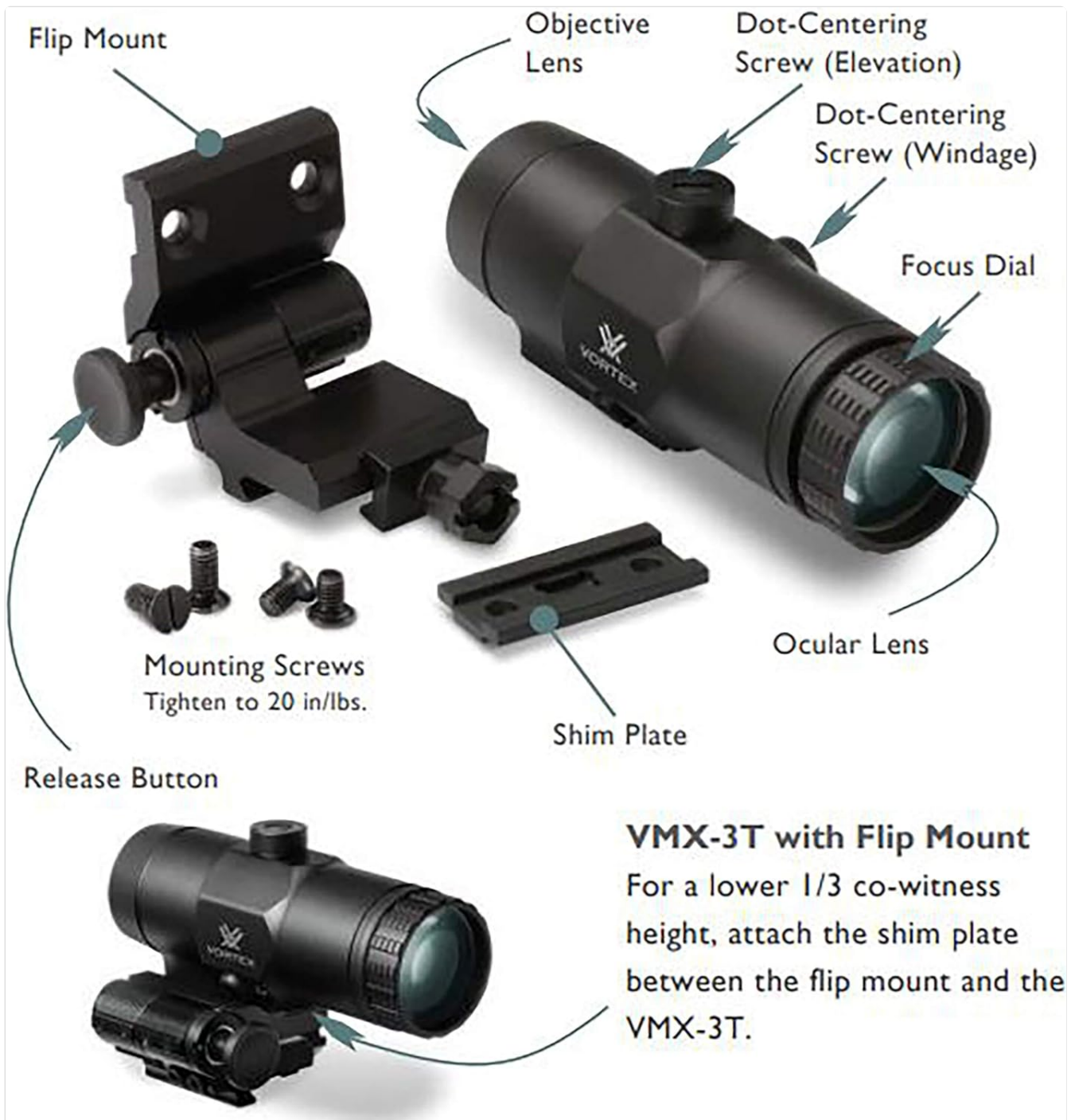
Image: Diagram illustrating the components of the VMX-3T with Flip Mount, including the objective lens, ocular lens, focus dial, dot-centering screws, flip mount, release button, mounting screws, and shim plate.
