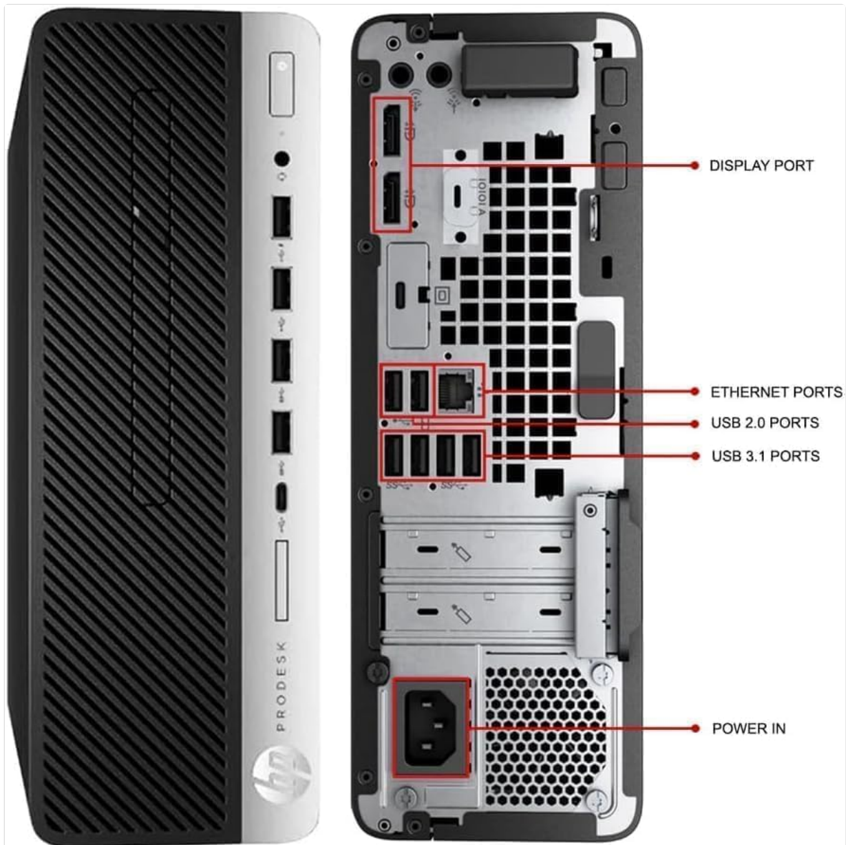
Image 3.1: Rear and side view of the HP ProDesk 600 G5 SFF with labeled ports.
