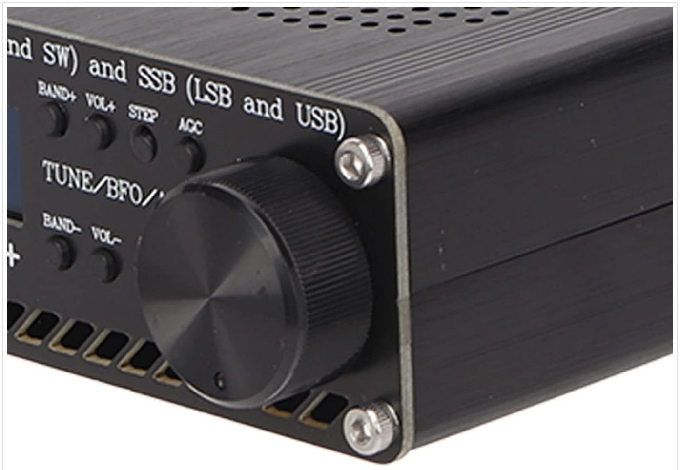
Figure 6: The large tuning knob for precise frequency adjustment.
