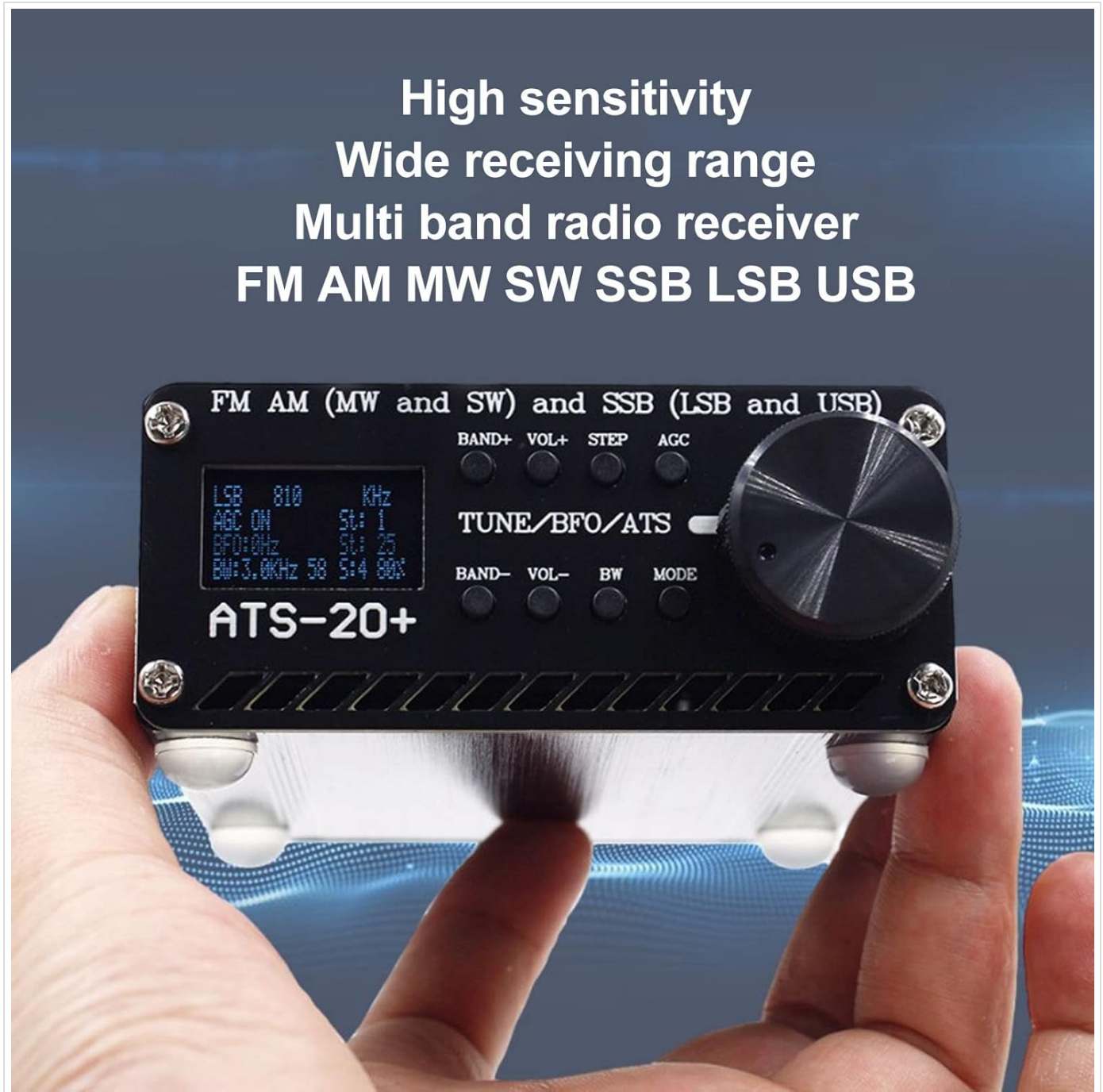
Figure 4: Detailed view of the radio's front panel, showing the display, tuning knob, and control buttons.
