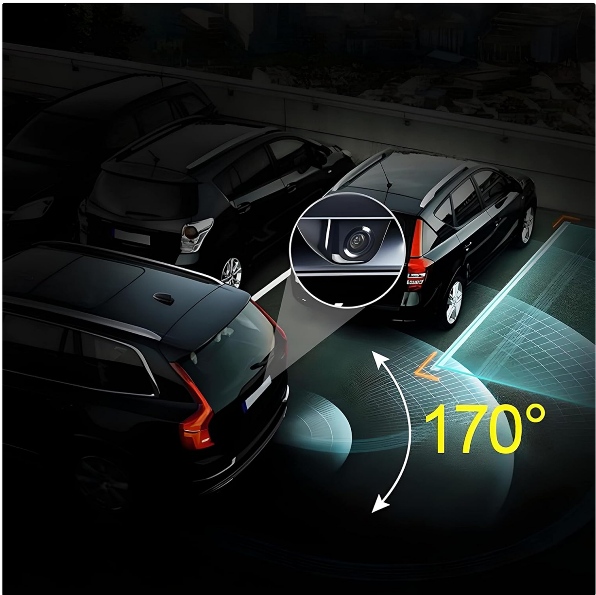
Figure 3: Illustration of the rear camera's wide 170-degree viewing angle, useful for monitoring the area behind the vehicle, especially during parking maneuvers.
