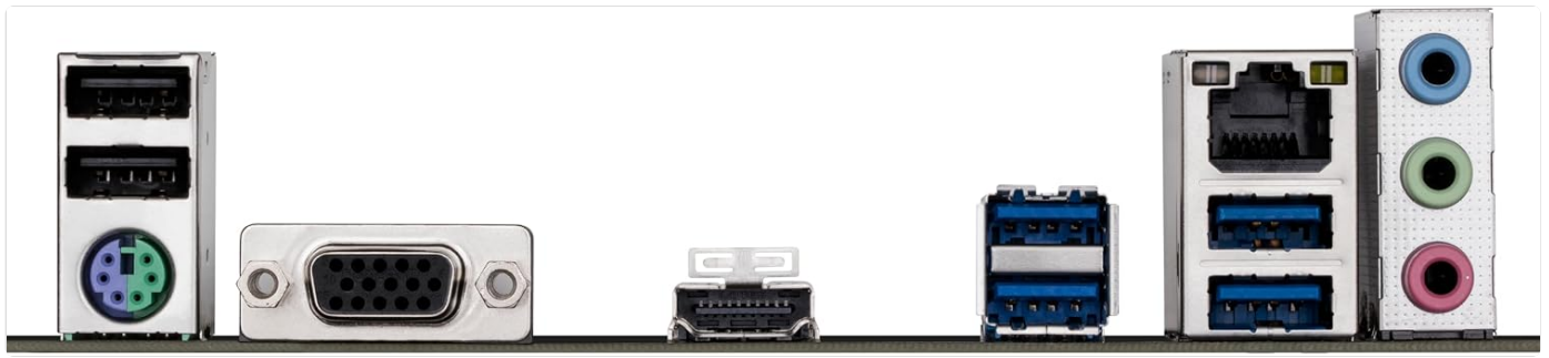
Figure 1.2: Rear I/O panel of the GIGABYTE A520M K V2 motherboard, displaying USB ports, video outputs, LAN port, and audio jacks.
