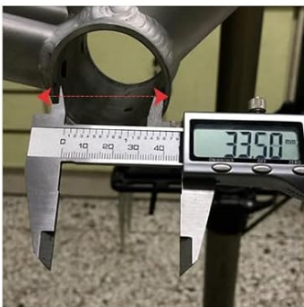
Figure 4.1: Compatibility check for the BAFANG mid-drive motor, including bottom bracket measurements and examples of incompatible bike setups (belt drive, coaster brake).
