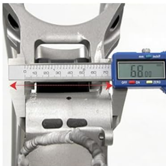
Figure 4.1: Compatibility check for the BAFANG mid-drive motor, including bottom bracket measurements and examples of incompatible bike setups (belt drive, coaster brake).
