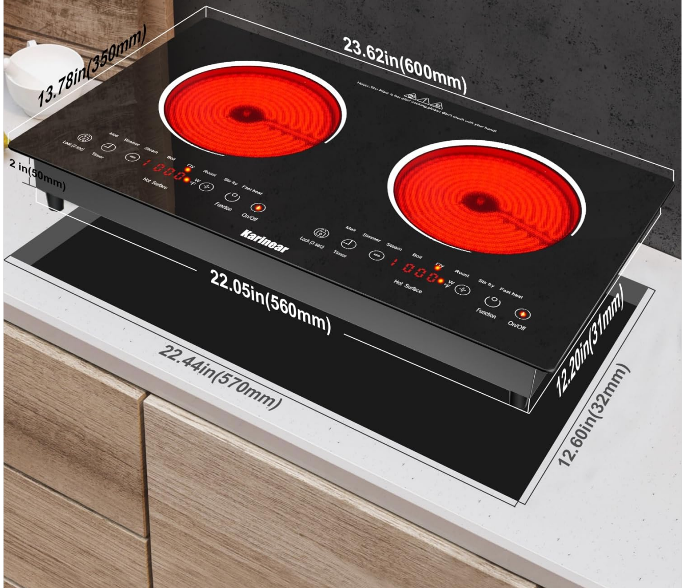
Figure 4.3: Detailed dimensions for built-in installation, including product and cut-out sizes.
