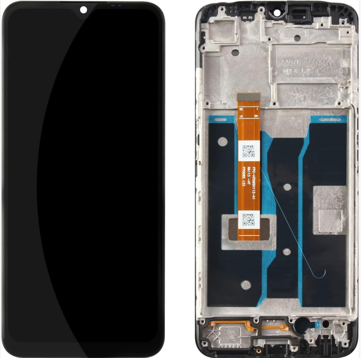
Image: Front view of the Oppo A16 LCD screen replacement, highlighting its 720x1600 pixel resolution and 6.52-inch size.
