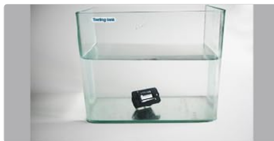
Figure 7: Water resistance test. The image shows the battery indicator submerged in a clear tank of water, demonstrating its IP68 waterproof rating.
