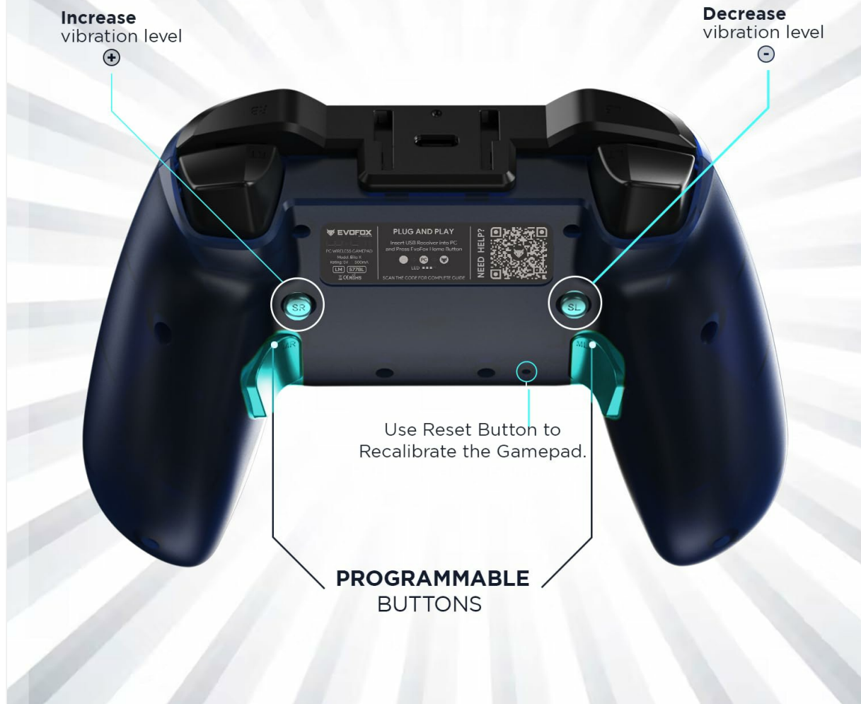
Image: The rear view of the controller, highlighting the programmable back buttons and dedicated buttons for adjusting vibration levels (increase/decrease).
