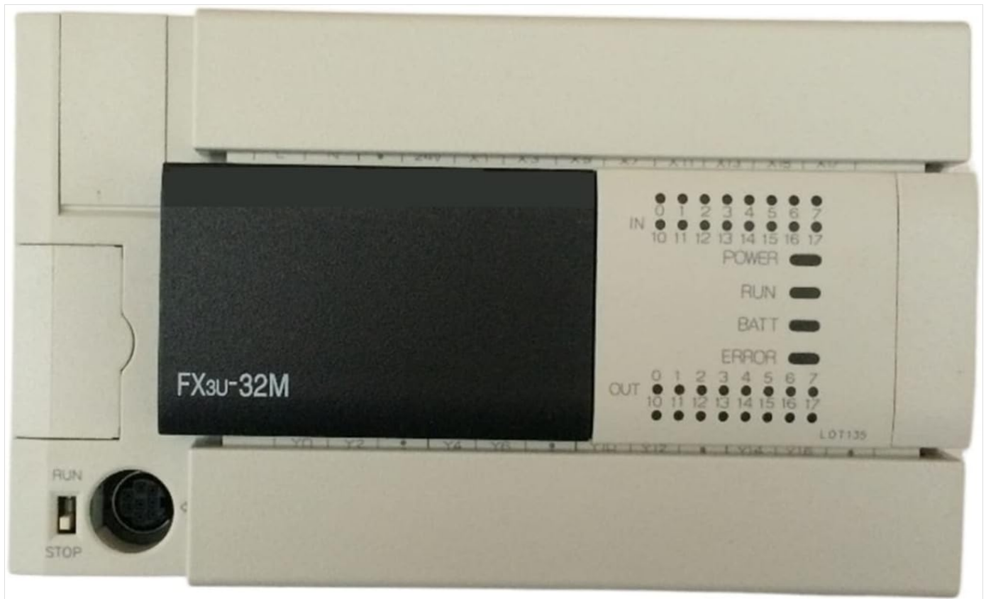
Figure 2: Front panel of the FX3U-32MR/ES-A PLC. This image displays the front panel, highlighting the input (IN) and output (OUT) status indicators (0-17), along with POWER, RUN, BATT, and ERROR indicators. The 'RUN' and 'STOP' switch is also visible on the left side.
