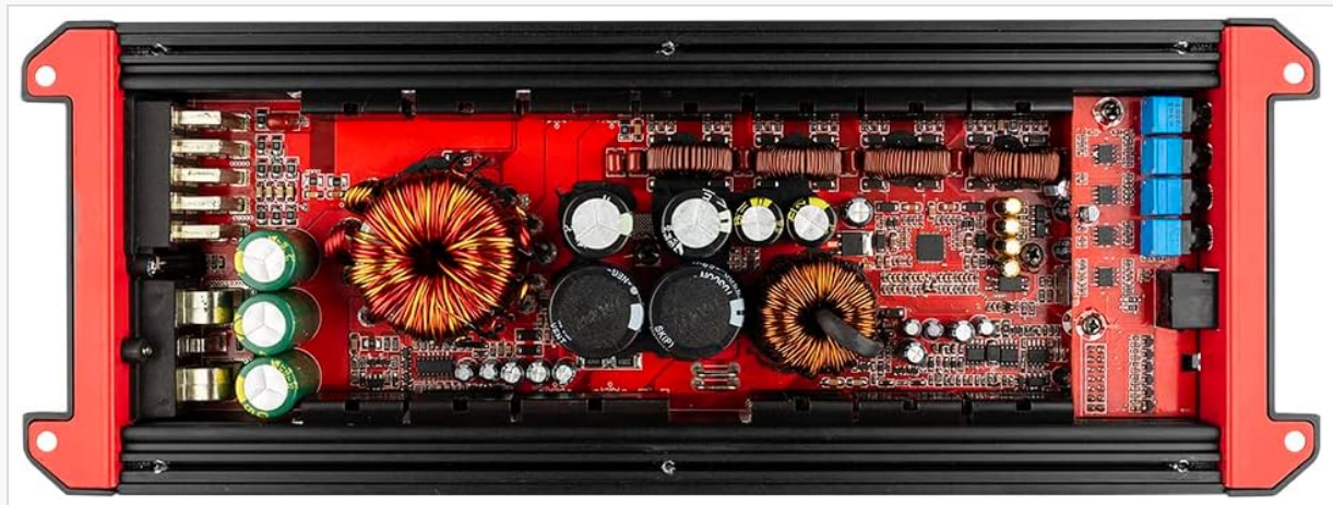
Figure 2: Power input and speaker output terminals. Ensure correct polarity and secure connections.
