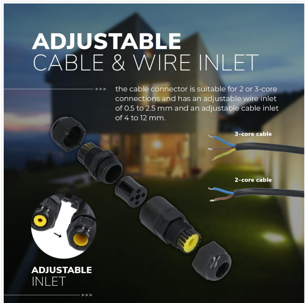
Figure 1: Adjustable Cable & Wire Inlet. The connector is suitable for 2-core or 3-core connections and has an adjustable wire inlet of 0.5 to 2.5 mm 2 and an adjustable cable inlet of 4 to 12 mm.
