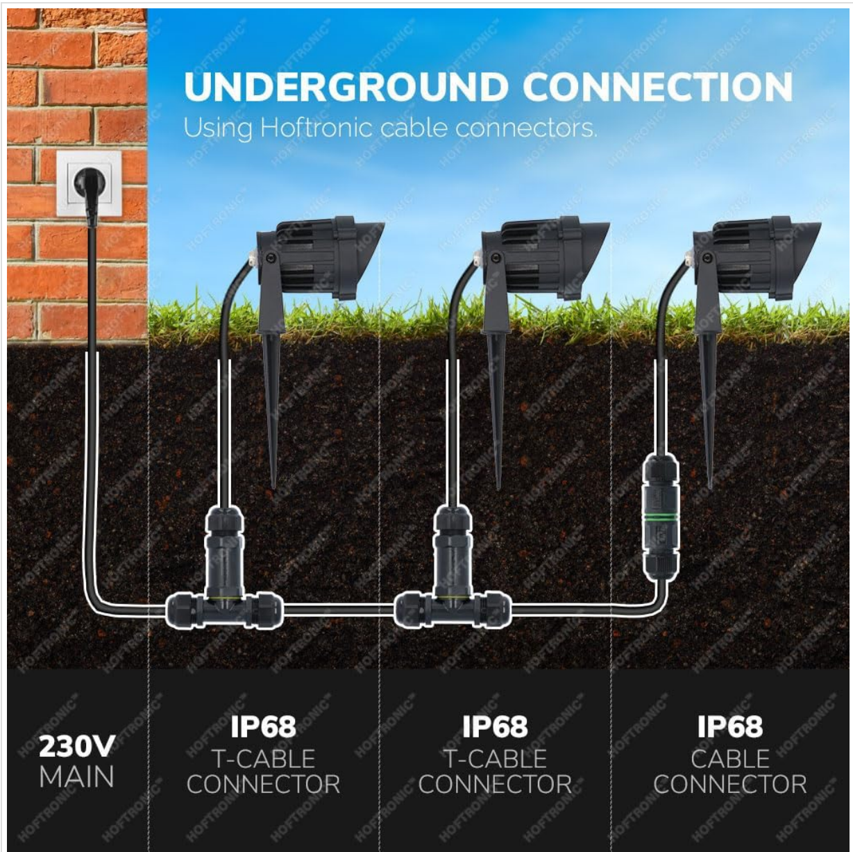
Figure 6: Underground Connection for Spotlights. An example of using HOFTRONIC cable connectors for underground wiring of garden spotlights.
