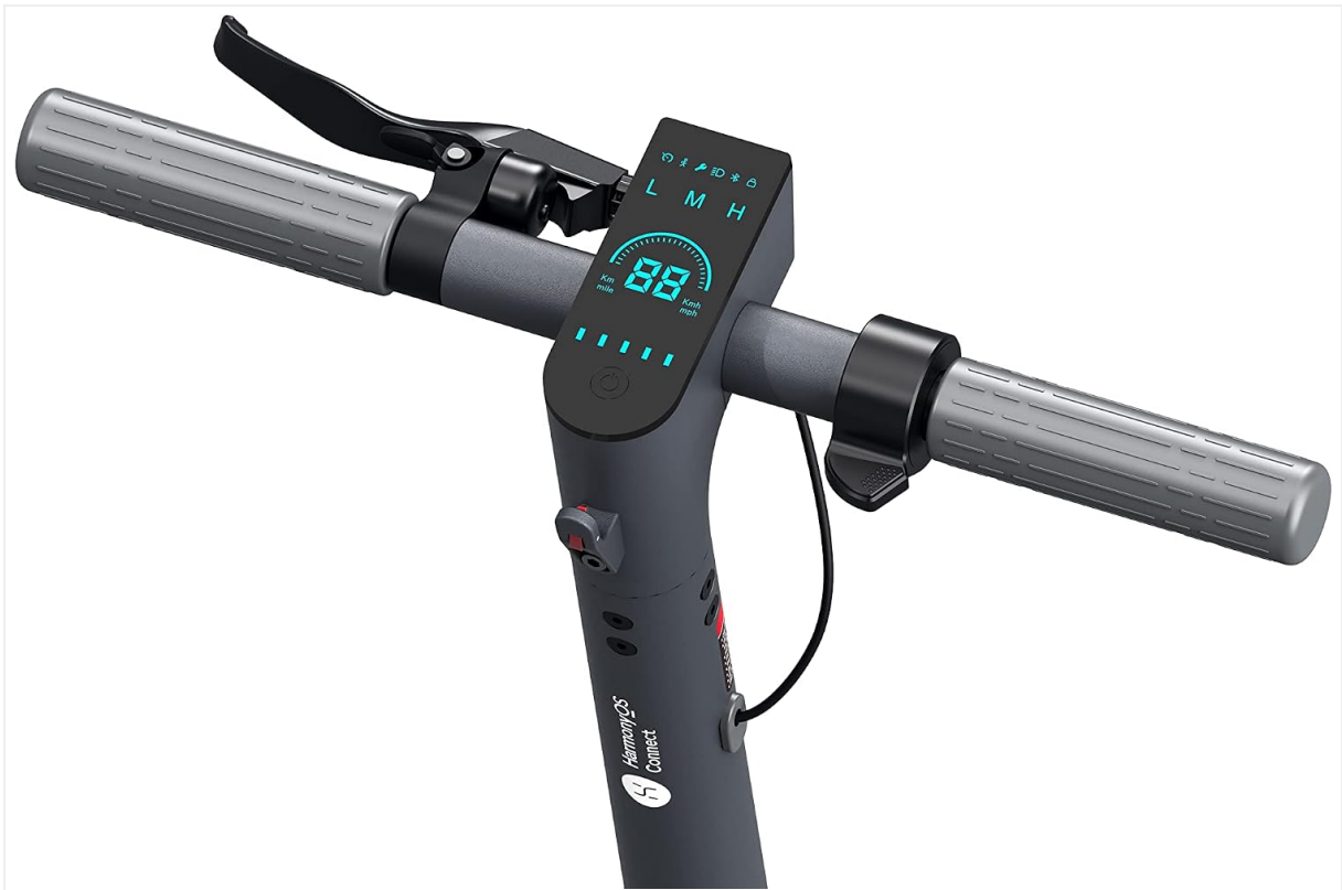
Figure 6.1: Close-up of the LEQISMART D12 Harmony Electric Scooter's handlebar display, showing speed, battery level, and riding mode indicators.
