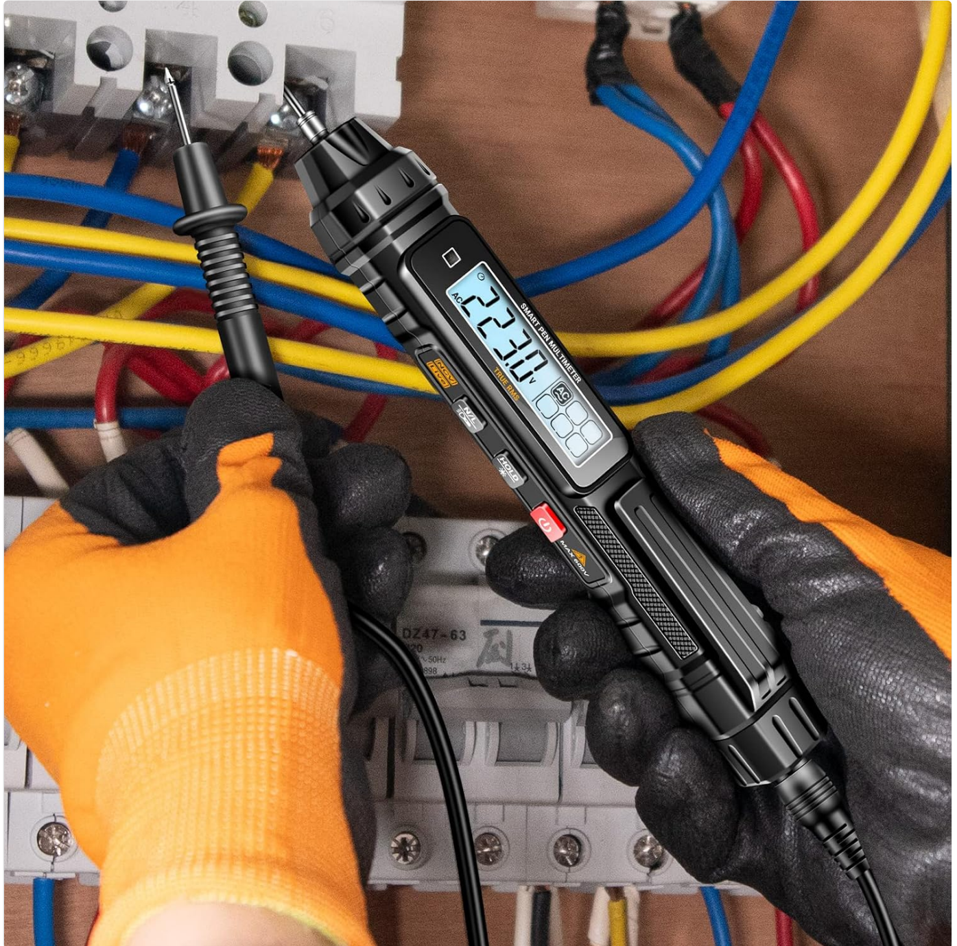
Figure 5.1: Measuring voltage with the ANENG A3005.
