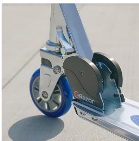
Image: The rear fender brake mechanism for stopping.
