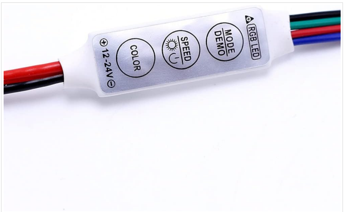
Figure 2: Close-up view of the controller's interface, highlighting the three control buttons: COLOR, SPEED, and MODE/DEMO, along with the 12-24V DC input label.
