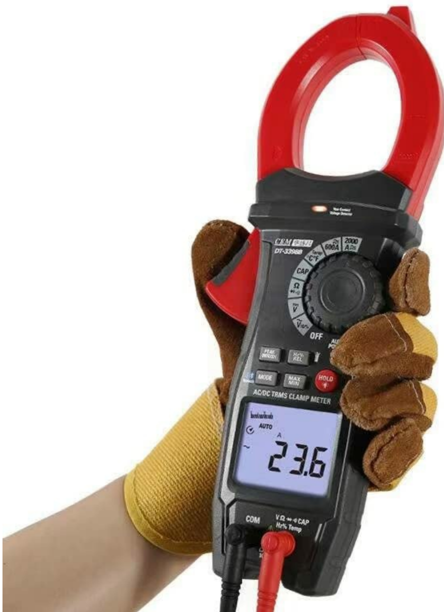
Figure 3: User holding the DT-3398B Clamp Meter, demonstrating proper grip and test lead connection points.
