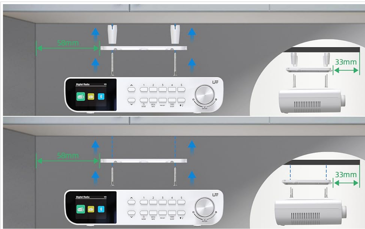
Image 5.2: Diagram illustrating the under-cabinet mounting process, showing screw placement and dimensions for secure installation.
