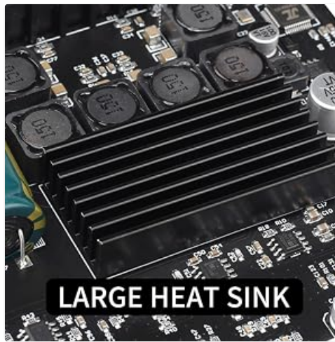
Image 4.1: Close-up view of the large heat sink on the ZK-AM100F amplifier board, essential for thermal management.
