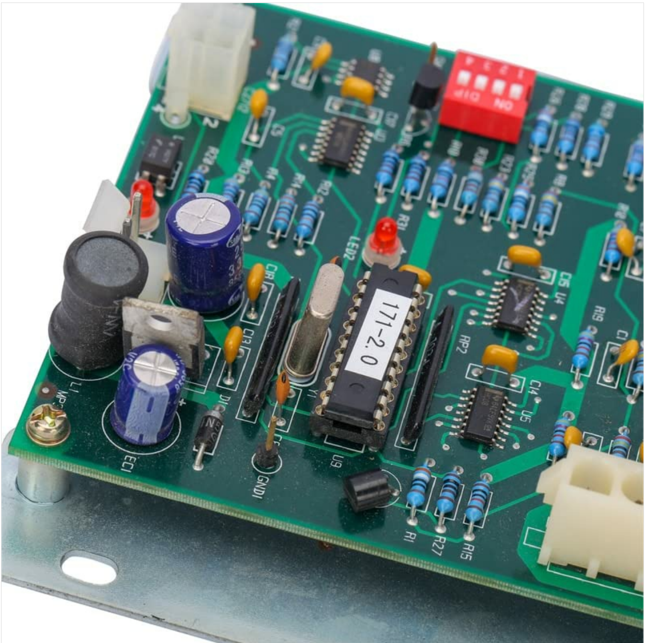
Figure 2.2: Detailed view of the central part of the control board, highlighting the main integrated circuit labeled "171-2.0" and surrounding capacitors, which are vital for the board's processing capabilities.
