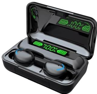
Before first use, fully charge the earbuds and the charging case. Place the earbuds into the charging case. Connect the USB charging cable to the case and a power source. The LED display on the case will show the charging progress for both the case and individual earbuds. A full charge is indicated by 100% on the display.
