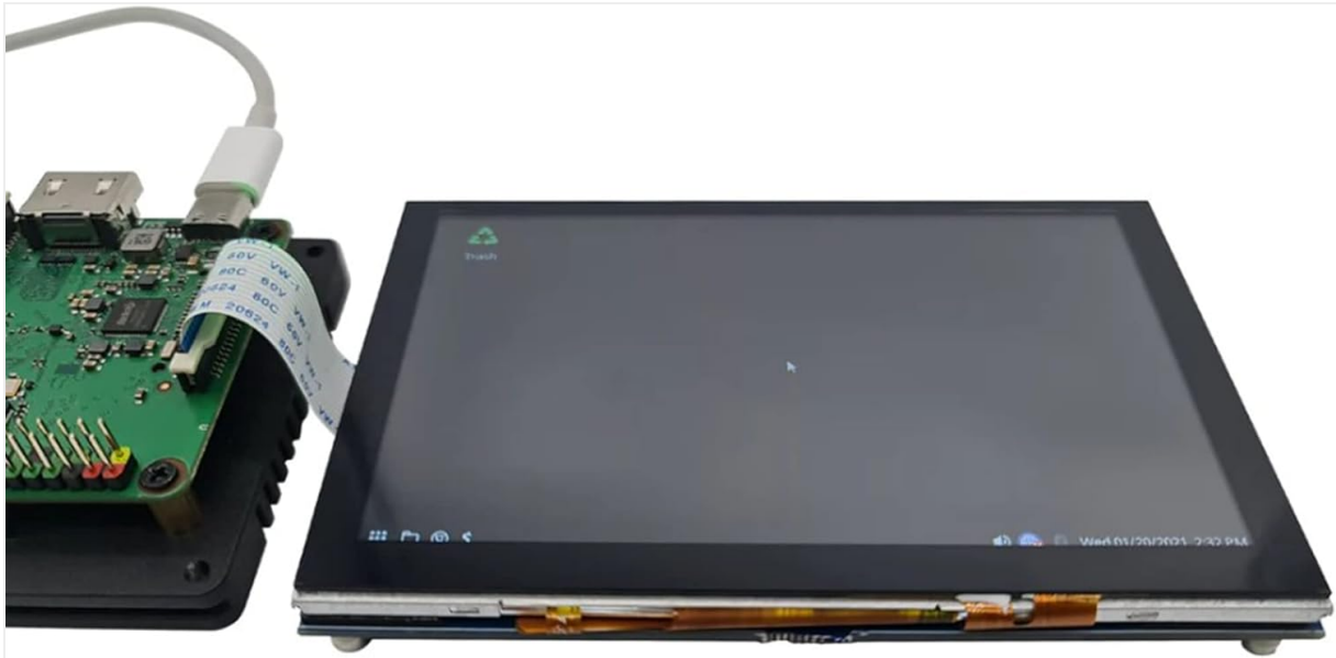
Image 2.1: The 5-inch Capacitive Touch Screen connected to a development board. The ribbon cable connects the display to the board's MIPI DSI port, and a USB cable provides power or data to the board.
