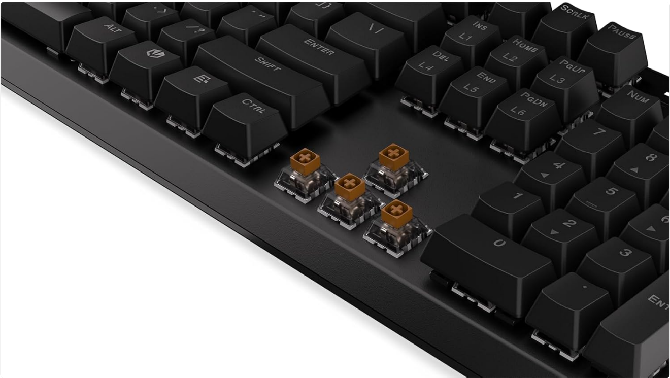
Image 4.2: A close-up view of the Kailh Box Brown mechanical switches, demonstrating the hot-swappable design.
