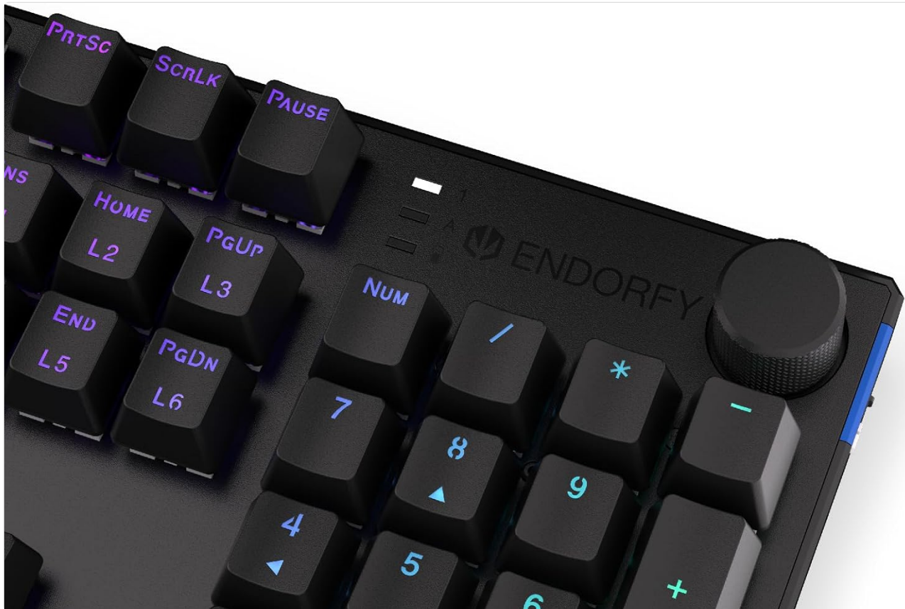
Image 4.1: Detail of the volume knob and status indicator lights, located on the upper right side of the keyboard.
