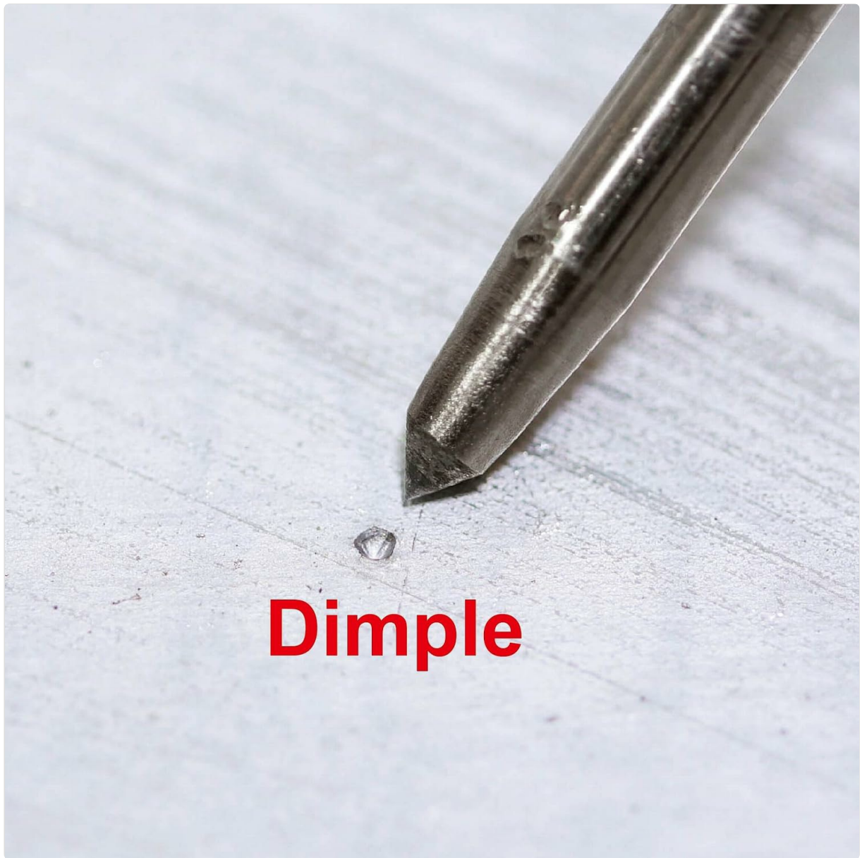
Figure 2: A clear dimple created by the automatic center punch on a surface.
