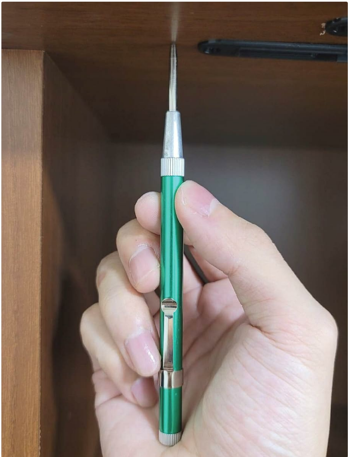
Figure 4: The knurled cap for adjusting the impact force (High/Low).
