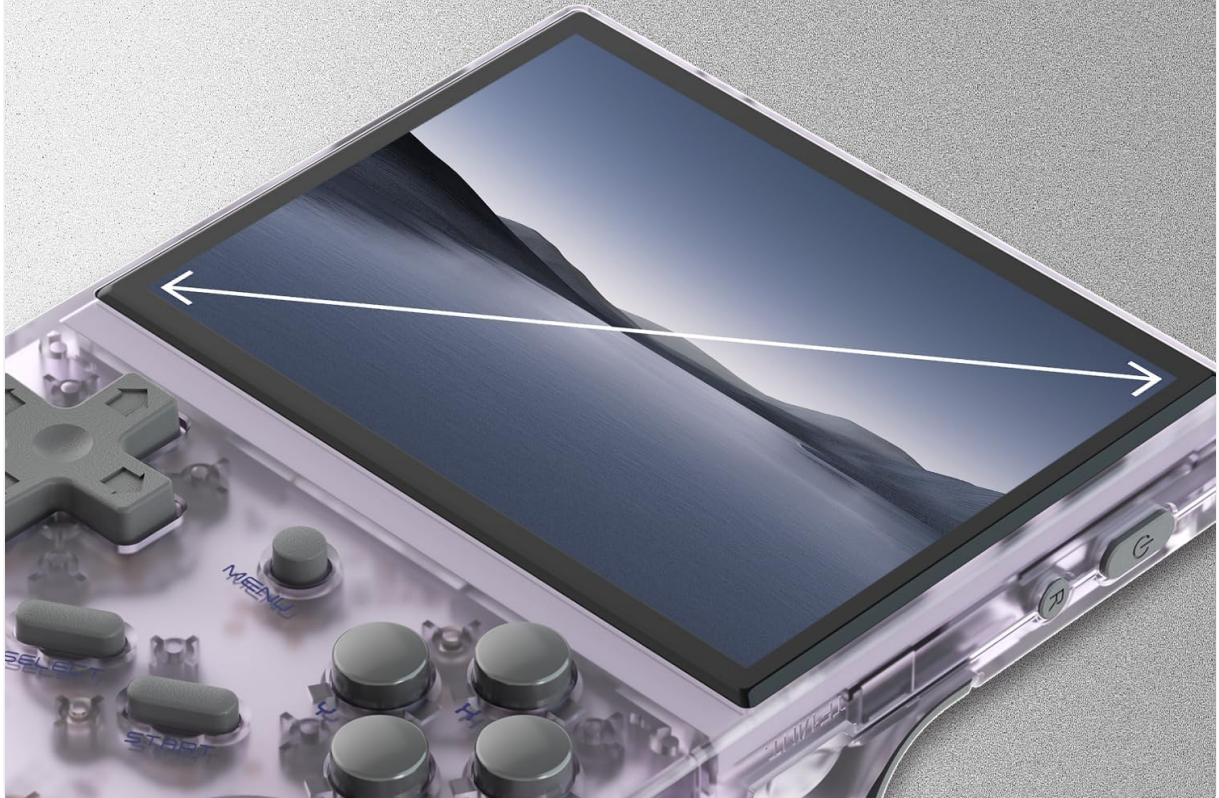
Figure 3.3: The 3.5-inch IPS screen, featuring 640x480 resolution, full viewing angle, and OCA full lamination for optimal clarity.
