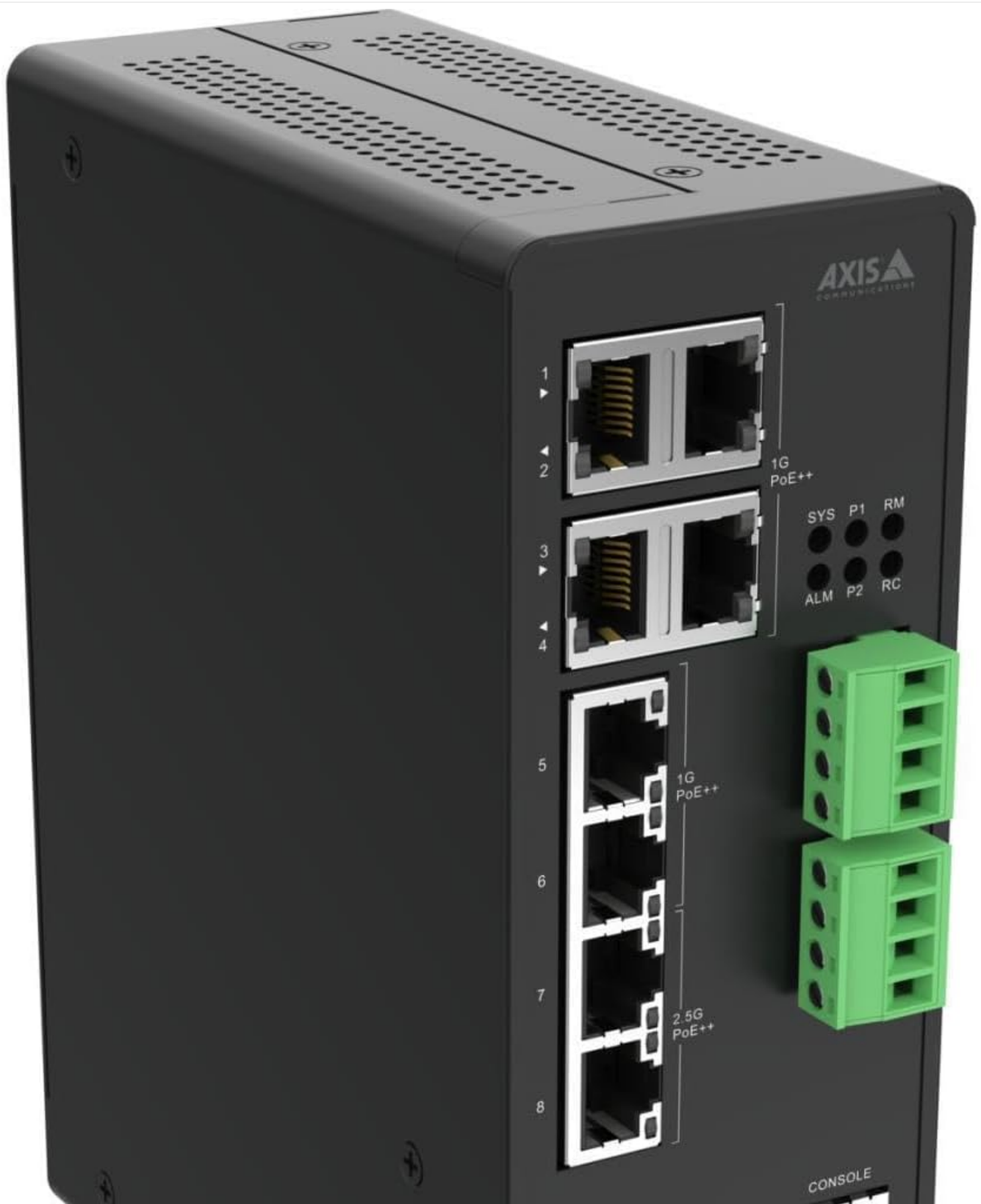
Figure 1: Front view of the AXIS D8208-R Industrial Switch. This image displays the front panel of the switch, highlighting the various Ethernet ports, power input terminals, LED indicators, and the console port. Ports 1-4 are 1G PoE++ ports, ports 5-8 include 1G and 2.5G PoE++ capabilities, and ports 9-10 are 10G SFP+ ports.
