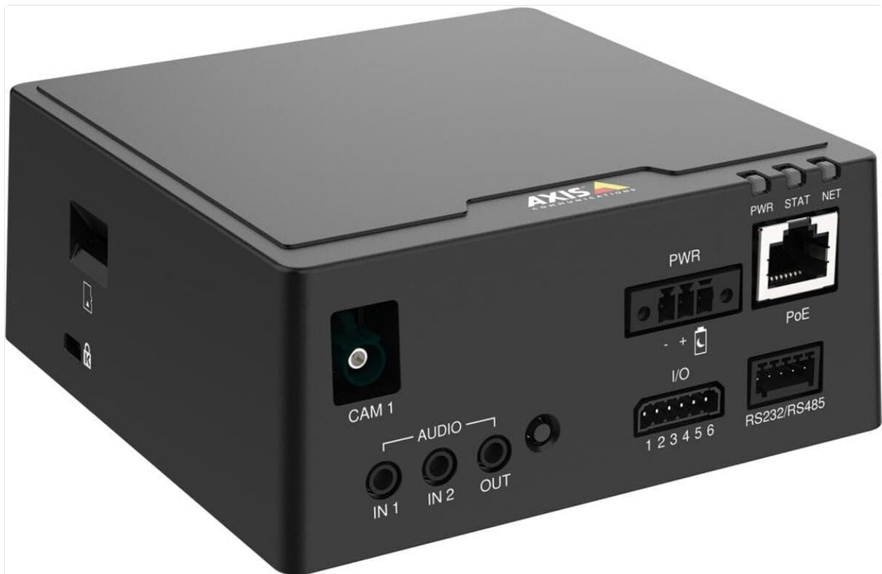
Figure 3: A different angled view of the AXIS F9111 Main Unit, further illustrating the layout of the various input/output ports and power/network connections for comprehensive system integration.
