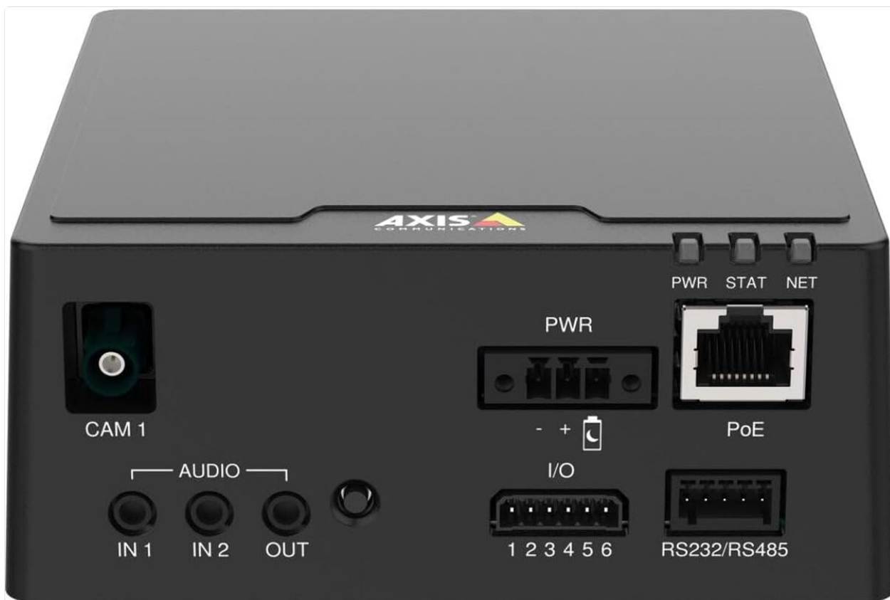
Figure 1: Top-down view of the AXIS F9111 Main Unit, highlighting the various connection ports and status indicators. From left to right, it shows the CAM 1 input, Audio IN/OUT, PWR input, I/O terminals, PoE Ethernet port, RS232/RS485 terminals, and PWR, STAT, NET LED indicators.
