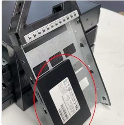
Figure 5.1: Illustrates the method for installing a 2.5-inch HDD into a drive tray.
