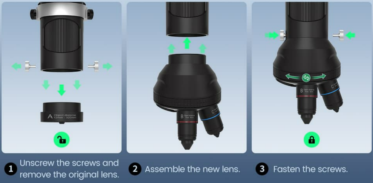
Image: Steps for safely switching lenses on the microscope.
