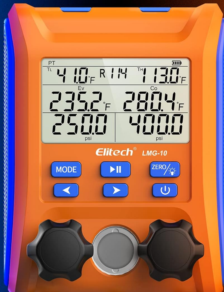
Image: A close-up of the Elitech LMG-10Plus display, illustrating how superheating (SH) and subcooling (SC) values are automatically calculated and shown alongside pressure and temperature readings.
