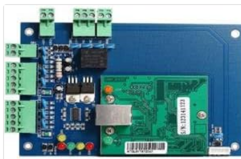
Figure 3: Access control panel circuit board.
