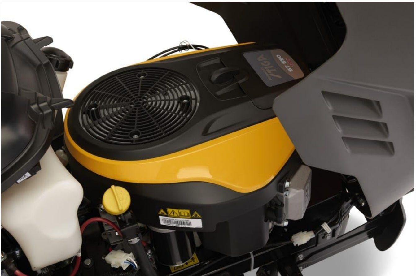
Figure 6: The engine compartment, showing the robust 586cc twin-cylinder engine.
