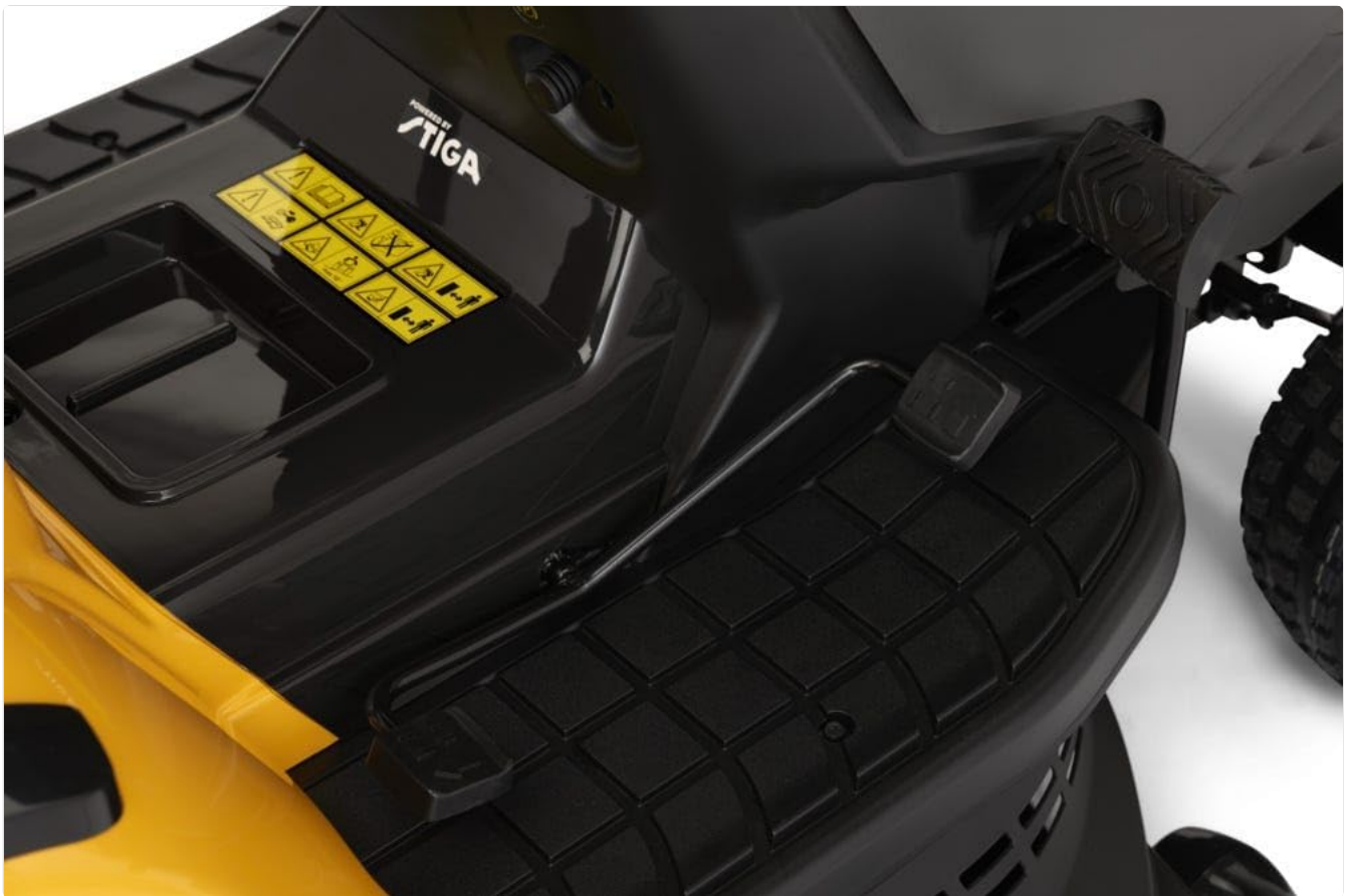
Figure 4: Foot pedals for controlling the hydrostatic transmission.
