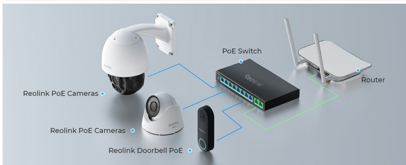
Figure 7: Connection diagram for cameras directly to the PoE switch and then to a router.
