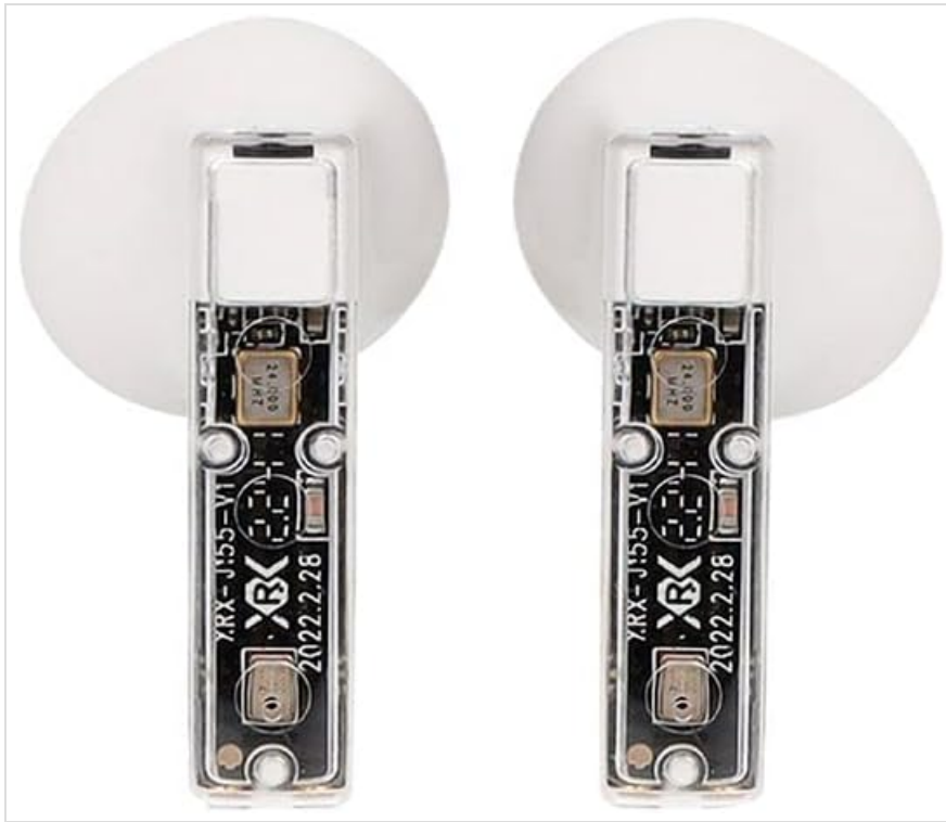
Image: A close-up view of the internal circuitry visible through the transparent casing of a Billboard Soul Clear TWS earbud.
