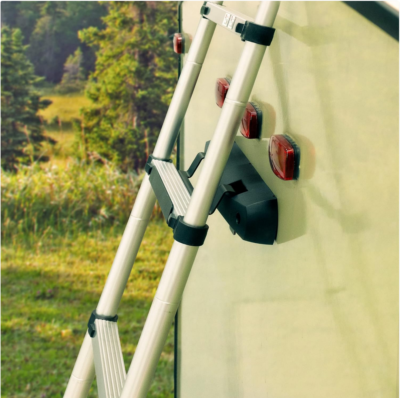
Image 4.1: A detailed view of the ladder's bracket, demonstrating its secure connection to a Lippert On-The-Go receiver on an RV.
