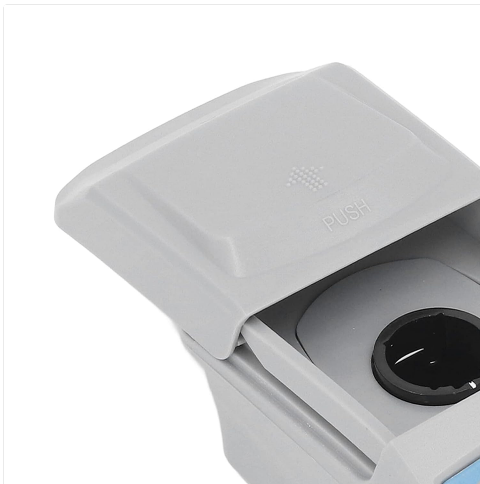
Figure 6.1: Detail of the sample chamber where the sample bottle is inserted.
